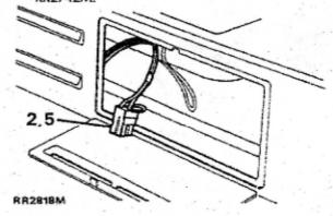
3. Remove the ABS warning light relay.
